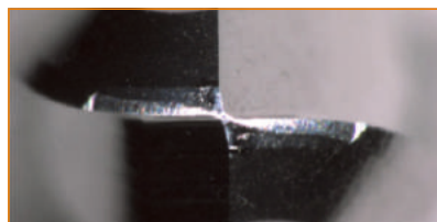
Fresa Rival ◀ Tool Wear: 0.095mm
