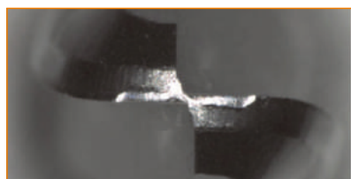
Fresa NS TOOL MRB230 R1x10 ◀ Tool Wear: 0.087mm
