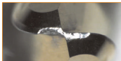
Fresa Rival ◀ Tool Wear: 0.136mm
